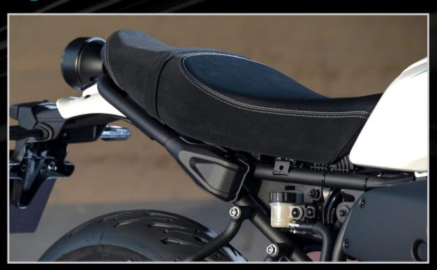
For easy manoeuvrability and sharp agility, the XSR700 runs with a slim, light steel backbone frame that is easily customisable due to its two piece subframe. Combined with its compact wheelbase and easy natured suspension system, this strong and light chassis gives a responsive and engaging ride.
