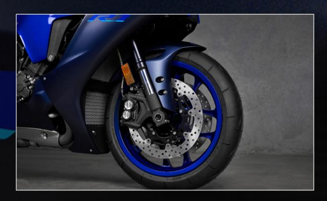
The R1 is equipped with high-specification 43mm KYB forks featuring laminated type damping valves. Together with the advanced rear shock this suspension system gives you a sensation of being connected directly to the road surface, making the R1 feel as if it is an extension of your body.
